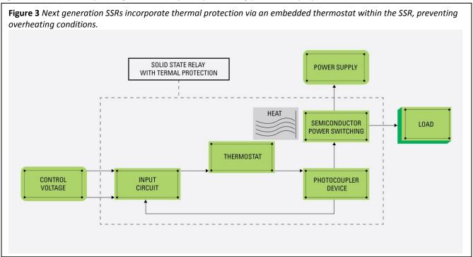
In addition to preventing overheating, the integrated thermal protection function can troubleshoot design issues in the system. It can help identify incorrect heat sinking capacity in the SSR or system, poor installation resulting in insufficient heat sinking contact, heat dissipation efficiency of the system, as well as other issues. This provides a valuable tool to the engineer responsible for the system's operation.
